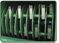
Rotary Grinder High speed grinder deforms engine vanes using hardened steel teeth
